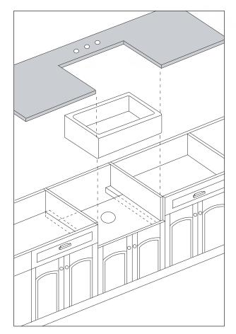
Once it is agreed upon, cut countertop accordingly. The actual sink is used as a template guide for each installation. After centering the sink and allowing for any faucets and backsplashes, use a pencil to outline the sink as your guide for the cutout, allowing for any reveal before the actual cutting.
